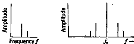
(a) Modulating function (b) Radio-frequency spectrum FIG. 2-1.—Sidebands produced by amplitude modulation.
