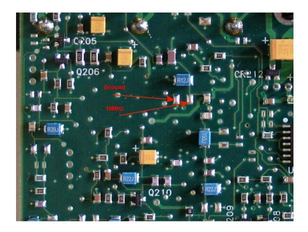
The pad indicated as 10MHz looks to be fed directly from the 10MHz doubler circuit. It has an amplitude of approx 1V P-P and will accept a relatively low impedance load, 1Kohm say, but on a 100MHz bandwidth scope is showing noticeable "ripple".
