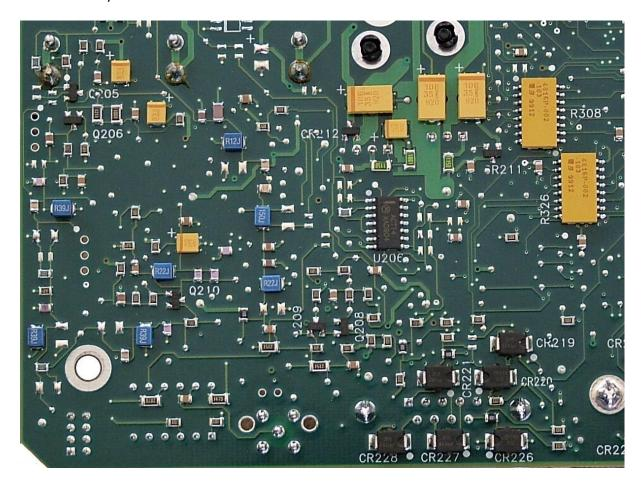
This picture shows the area of the bottom side of the dismantled pc board where the modifications have to be done. As the soldering of 0805 and SOT23 SMD components has to be done a suitable fine soldering iron and a tweezers will be necessary. The next photo shows the pc board and the position of the referred components.
